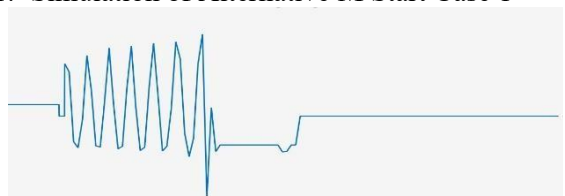
Fig 4. Voltage response during the starting of motor M532FN11
